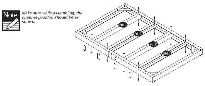
$5. \ \mbox{Fix}$  the channel (F02C) into the frame with screws as shown. See Fig.
