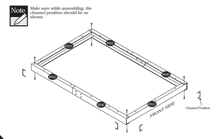
$3. \ \mbox{Fix}$  the L-angle (F03) to the channel at all the four corners to make a perfect frame. See Fig.
