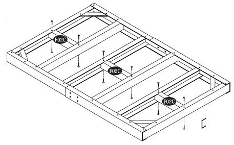
$\ensuremath{6}.$  Assemble the U-Channel bases on top of the foundation as shown in Figure.
