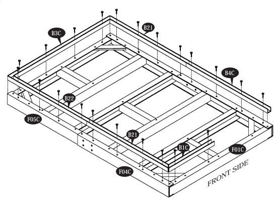
7a. After completing the assembly of shed place exterior grade CDX  $3/4\mbox{''}$  (19mm) plywood inside the foundation. See fig.
